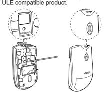
The registration process takes about 90 seconds to complete. When this registration process completes, the green LED light on the sensor will remain steadily on for approximately two seconds then, will turn off.
